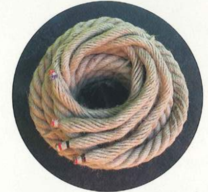
FIRST, GLUE THE ENDS TO PREVENT FRAYING. TYING COLORED STRING TO EACH END HELPS KEEP TRACK.
