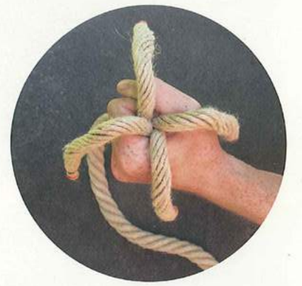
GRAB THE STRANDS WITH YOUR FIST AND NEATLY LAY THE FOUR STRANDS OVER YOUR HAND, LIKE SO.
