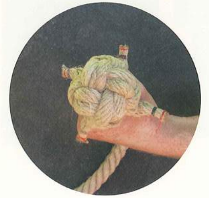
ONCE DOUBLED, PUSH EACH STRAND DOWN THROUGH AT THE END. WORK THE ENDS TIGHT AND SHAPE INTO A TIDY BALL.
